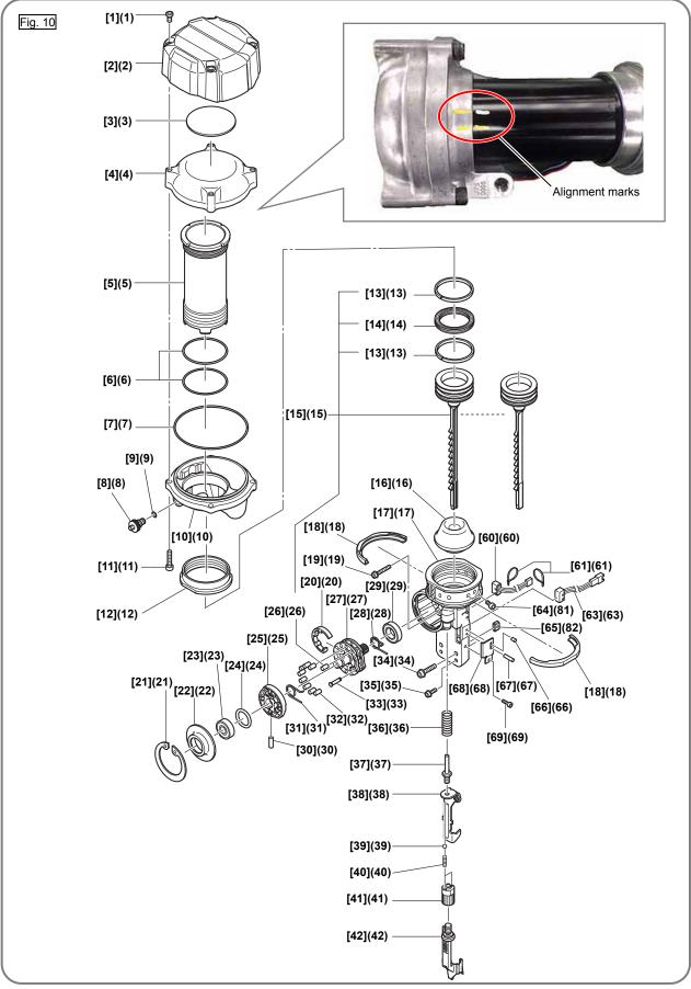
• Remove the valve core from the Chamber Base **[10](10)** by using a commercial valve core tool. (See Fig. 11.)
