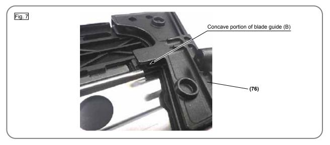
• Insert the protrusion of Nail Rail (C) (87) into the nail head inlet of Blade Guide (B) (76).
