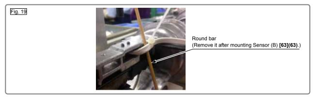
• Apply Molub-Alloy 777-1 grease to the following area on the Nose **[17](17)** and then mount Pushing Lever (B) **[38](38)**.
