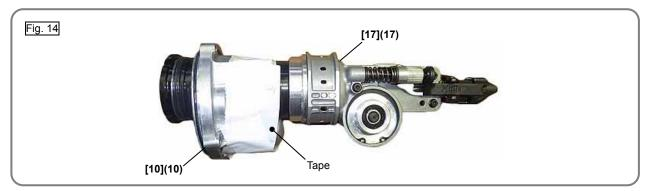
• Fix the hexagonal portion of the J-400 special socket. Fit the claws of the J-400 special socket in the notches on the end surface of the Cylinder [5](5). Loosen the Special Nut M58 [12](12) and turn the Nose [17](17) to remove it from the Cylinder [5](5).
