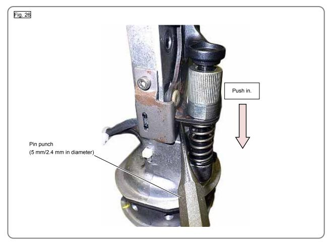
If the LED light remains turned off when inserting a pin punch of 5 mm in diameter during the operation check of Sensor (B) [63](63) or if the LED light turns on when inserting a pin punch of 2.4 mm in diameter, Pushing Lever (B) [38](38), Blade Plate (P) [68](38) or Sensor (B) [63](63) may be damaged or deformed. Check and replace the damaged or deformed part and then perform the operation check of Sensor (B) [63](63) again.
